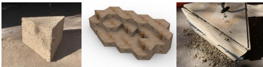
Figure 10. (left) Hempcrete prototype. (center) Plan for constructing seating in outdoor classroom/amphitheatre. (right) Hempcrete casting process, central to an upcoming build-a-thon community activation. Prototypes: Brandon Buerk, BFA Design student, guided by Kate Catterall and Alyson Beaton.
